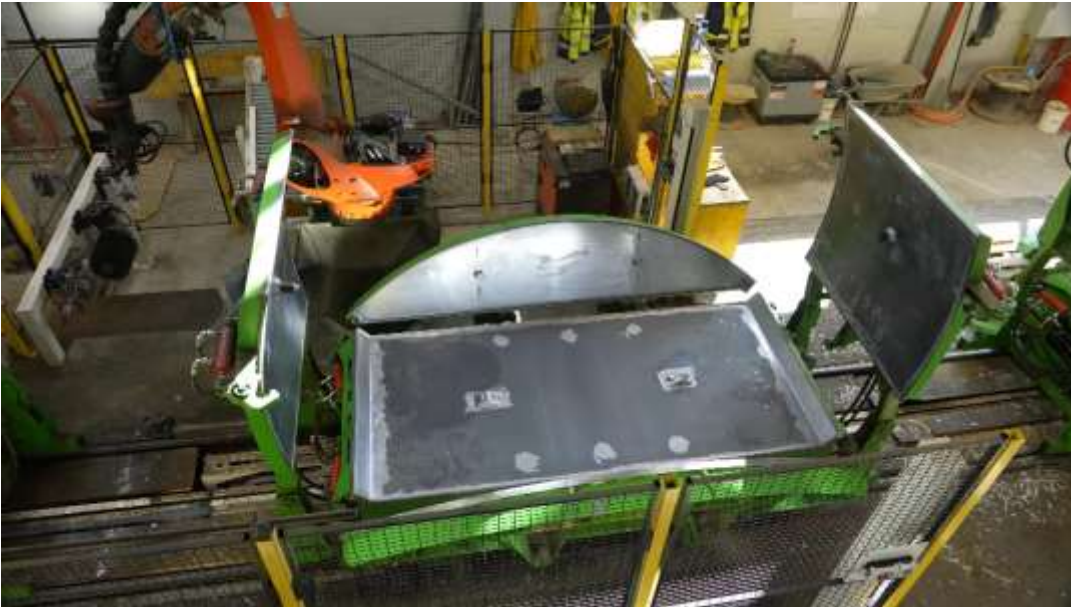
MOULD CLEANING & OILING (with tool change)
