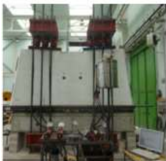
Figure 1.2. Push test on segment S1-S2. Load on the single joint to test
