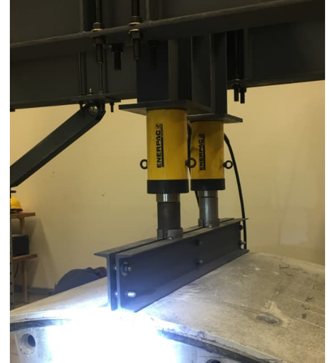
Hydraulic rams with 900 kN max. loading capacity, each
