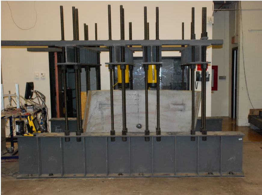
Load Frame for compression testing
