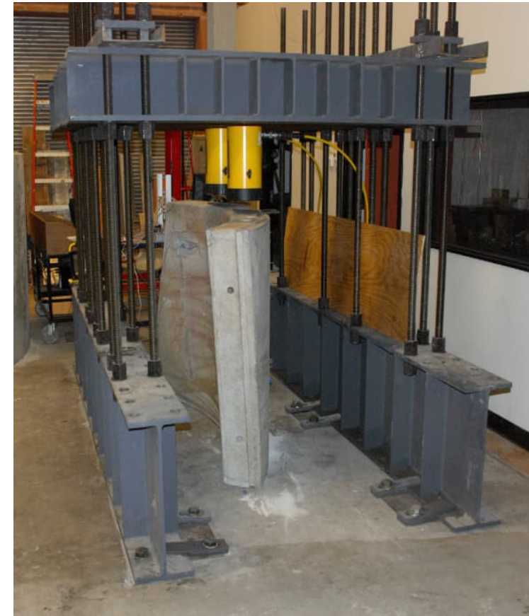
Hydraulic rams with 200 kips max. loading capacity, each
